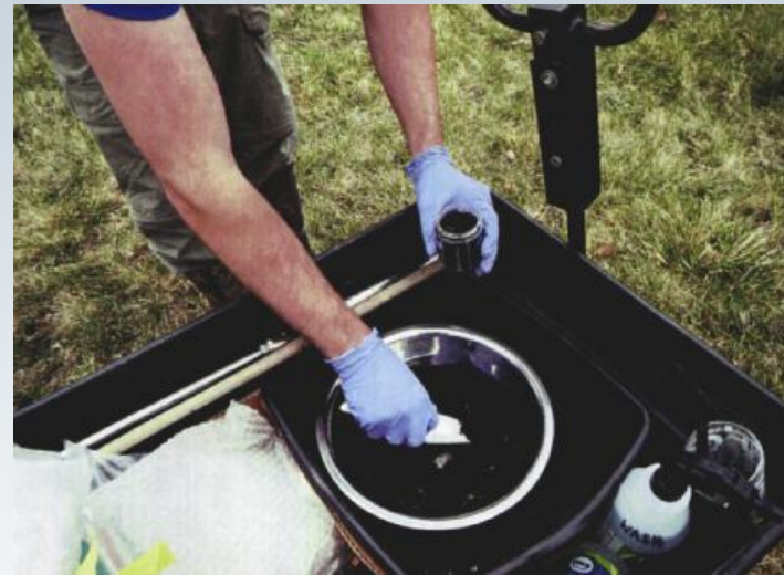
Collecting soil samples to analyze for metals and polycyclic aromatic hydrocarbons.
