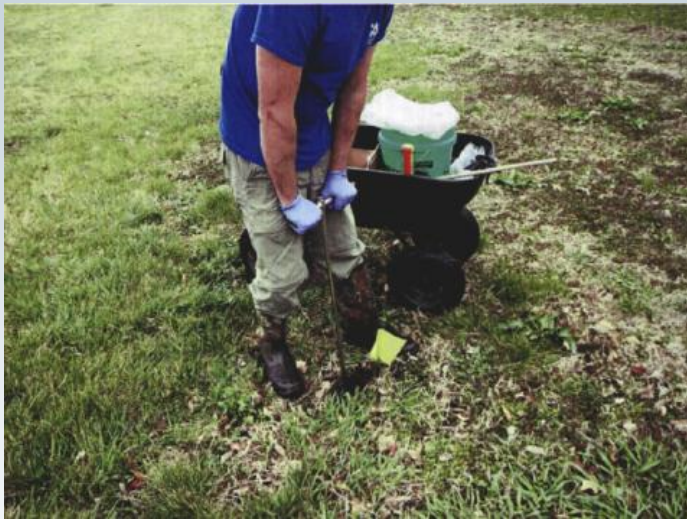
Collecting soil samples to analyze for metals and polycyclic aromatic hydrocarbons.
